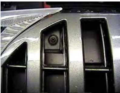
Hole location for the BX8869.
