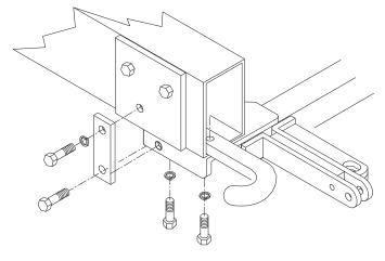
4. Take the flat braces (Items 2 & 3) and fasten them to each side of the frame and to the side of the baseplate. Use the 1/2 x 1 3/4" bolts, lock washers and nuts (Items 4,5,6) to fasten the brace to the baseplate. Use the existing 14mm bolt to fasten the brace to the frame of the vehicle. Be sure to use Loctite with each bolt. Once all bolts have been started, tighten according to the torque chart in the General Instruction Sheet.
