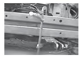
10. Place the baseplate up to the vehicle so the front holes in the brace are centered to the bottom of the metal bumper and the side plates are on the outside of the frame. Clamp the baseplate to the bumper.
