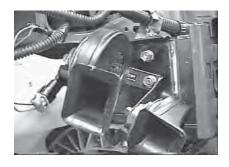
12. Use the 3/8" Whiz nut and fasten the horn to the lower bolt on the side plate.
