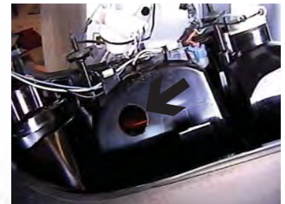
Location for the BX8869, top view of driver's side tail light assembly.
