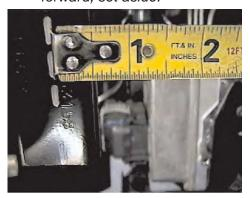
16. Locate front washer reservoir bracket on the passenger's side, measure 1/2" from bracket edge and up to bumper bracket, remove this portion of bracket with the reciprocating saw This will prepare area for baseplate installation.
