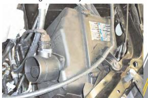
Using the phillips screw driver, remove the two phillips screws from filter assembly, disconnect electrical plug and set cover aside.
