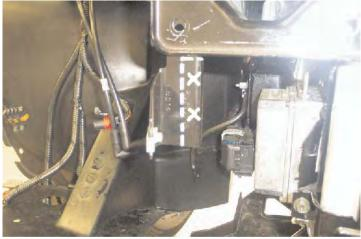
**13.** Remove the metric bolt from the lower bracket of small radiator from the back side of metal bumper and tie up out of the way.
