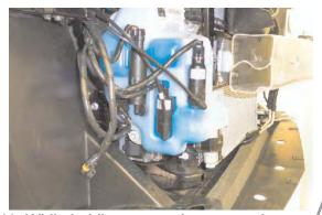
11. While holding reservoir, remove the metric bolt between wheel well and reservoir with the 10MM socket. Unplug electrical lines, disconnect and plug fluid lines, set reservoir aside.
