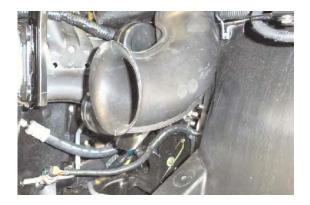
7. Using the 10MM socket, remove two metric bolt from filter assembly, lift assembly tube end out of fender and engine compartment, set aside.
