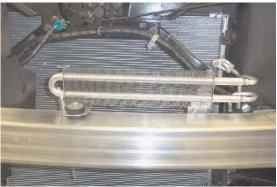
**12.** Using the 10MM socket remove the metric bolt from small radiator on the top side of metal bumper.
