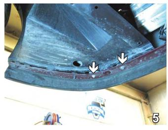
5. Using the 7mm socket, remove two metric bolts from the lower outside edge of the fascia. Do this to both sides of the vehicle. Set bolts aside to be reinstalled later.
