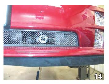
14. Hold the fascia up to its original location. Mark and trim the grille with the diagonal cutters as necessary for the attachment tabs, convenience links and electrical rods to come through. Reinstall the engine compartment covers and fascia.
