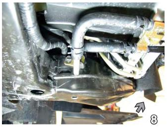
8. Just behind the grille, attached to the fascia, remove one Christmas tree pushpin from the air dam to loosen the air dam from the fascia (do not remove). Do this to both sides of the vehicle. Pull the fascia forward to remove. Set pushpins and fascia aside to be reinstalled later.
