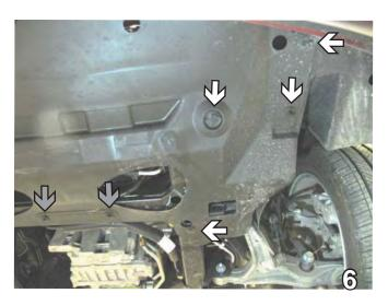
6. Remove four pushpins from the outer edge of the belly pan (see white arrows). Do this to both sides of the vehicle. Remove two pushpins from the center of the belly pan (see grey arrows). Remove belly pan. Set pushpins and belly pan aside to be reinstalled later.
