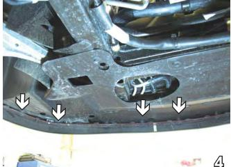
Remove eight pushpins from the bottom of fascia (driver's side shown). Do this to both sides of the vehicle. Set pushpins aside to be reinstalled later.
