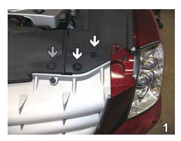
Above the grille, remove two pushpins (see white arrows) from the outer edge of the black plastic engine compartment cover. Remove cover and set aside with pushpins to be reinstalled later. Remove one pushpin from the center engine compartment cover (see grey arrow). Do this to both sides of the vehicle. Set cover and pushpins aside to be reinstalled later.
