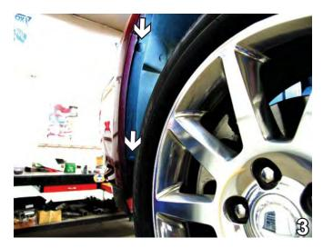
Just forward of the front tire, inside the wheel well, remove two pushpins. Do this to both sides of the vehicle. Set pushpins aside to be reinstalled later.
