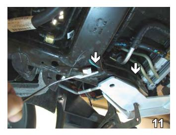
11. Insert 1/2-13 nut plate through one of the frame openings (see white arrows) and align to drilled holes. Insert the 1 1/2-13 x 1 1/2" hex bolts and 1/2" lock washers. Align with nut plates and tighten with the 3/4" socket. Trim nut plate wires. Do this to both sides of the vehicle.
