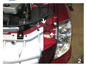
On the upper corner of grille, remove one pushpin (see grey arrow). Remove two pushpins from the upper corner of fascia (see white arrows). Do this to both sides of the vehicle. Set pushpins aside to be reinstalled later.
