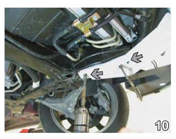
Using the baseplate as a template, drill two holes into the bottom of the frame with the 17/32" drill bit. Do this to both sides of the vehicle.
