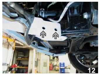
12. Using the baseplate as a template, drill two holes into the side of the frame with the 17/32" drill bit. Insert 1/2-13 nut plate through one of the frame openings and align to drilled holes. Insert the 1 1/2-13 x 1 1/2" hex bolts and 1/2" lock washers. Align with nut plates and tighten with the 3/4" socket. Trim nut plate wires. Do this to both sides of the vehicle.
