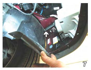
7. Using the 10mm socket, remove one hex bolt (see white arrow) and loosen (do not remove) stud nut just forward of the front tire inside the fender well. Do this to both sides of the vehicle. Set bolts aside to be reinstalled later.
