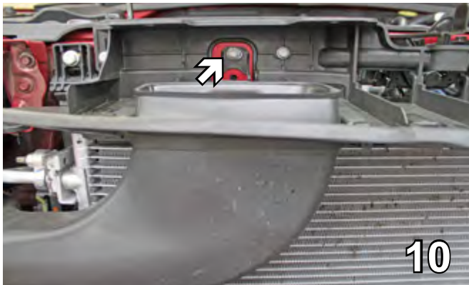
10. On the passenger side using a 10MM socket, remove the metric bolt from the top of the air baffle. Set the bolt aside to be reinstalled later.
