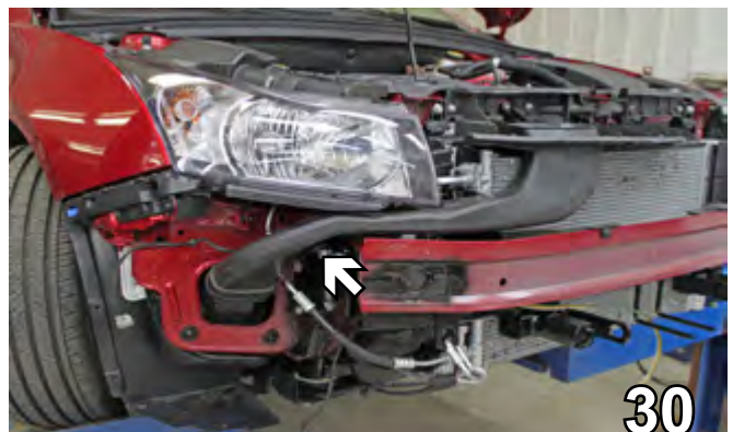
30. Reattach the upper portion of the air baffle.
