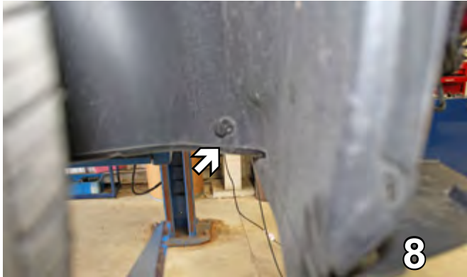
8. On the passenger side, inside the wheel well, remove one push pin. Set push pin aside to be reinstalled later.
