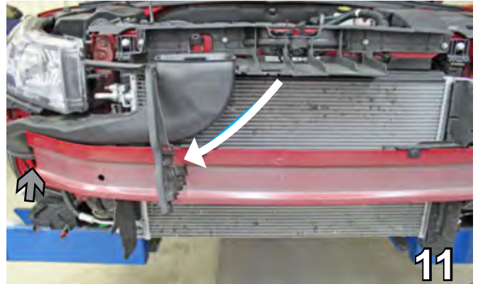
11. On the passenger side move the plastic ledge from the top of the tube (white arrow). Below the headlight, detach the air baffle from the bottom section of the tube (gray arrow). Set aside to be reinstalled later.
