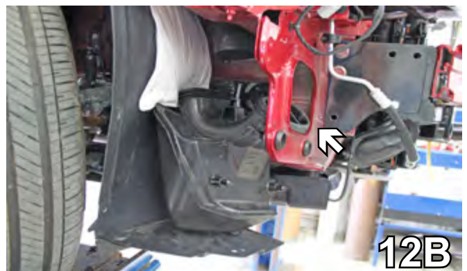
11. On the passenger side, push the air baffle back and slide it down to remove. Set aside to be reinstalled later.
