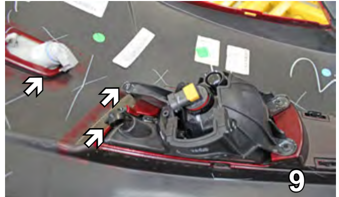
9. Inside the fascia on the driver side, unplug the side lamp, temperature sensor and fog lights. On the passenger side, unplug the side lamp and the fog lights.
