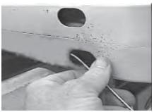
10. Insert 1/2" nut plate through slots in the front of metal bumper. Loctite bolts and tighten according to the chart in the General Instruction Sheet.
