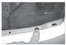
2. Remove the screws from the top of the bumper facia.
