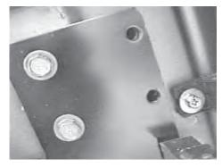
11. Center punch and drill 3/8" holes for remaining two holes. Use 3/8" hardware and tighten. Use loctite.
