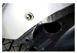
**2.** Just forward of front tire, on fascia corner, remove one screw with the phillips screw driver, both sides.
