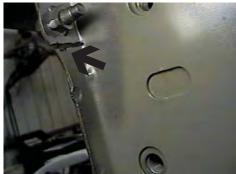
**5.** Cut frame ribbing, just forward of tow hook, with the hack saw. Using the 14MM socket, remove the three metric bolts from tie down bracket and set aside. Factory tie down bracket will **not** be reinstalled.
