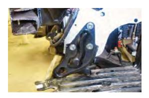
Remove the tie down bracket with the 14MM socket, both sides. Tie down brackets will not be reinstalled.
