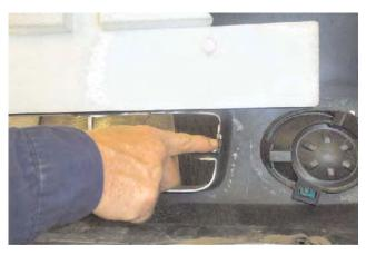
**16.** Cut and remove clip tab at the end of grill opening on both ends, flush with the back edge of grill's main body. Reinstall fascia.
