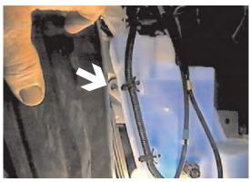
9. Remove metric bolt from between wheel well and washer reservoir using the 10MM socket,, pull reservoir down, unplug electrical connections, disconnect and plug water lines, set aside.
