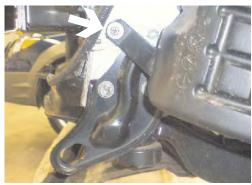
6. Remove metric bolt from air baffle, just above tie down bracket on driver's side and metric bolt between back side of baffle and wheel well cover
