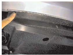
5. Remove the six push pins from the lower, middle edge of fascia, pull fascia forward and set aside.
