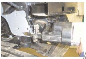
**11.** Mark webbing forward of tie down bracket area just below upper bolt (white arrow, left photo) and down flush with outside edge of frame with the reciprocating saw, both sides,
