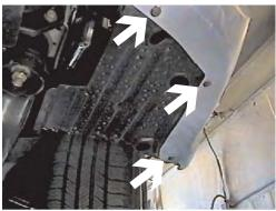
4. Forward of front tires, on lower edge of fascia, are three Phillips head screws to remove with the Phillips screw driver, both sides.
