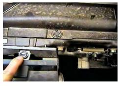
2. Pull the top edge of grill forward, just to the left of hood latch and remove push pin.
