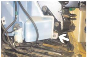
7. Using the 10MM socket, remove metric bolt from front washer reservoir on the passenger's side with the 10MM socket.
