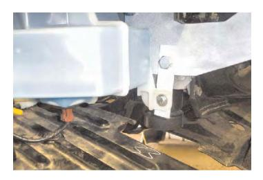
14. Install washer reservoir with existing bolts on the two back bolt locations and the 1/4-20 x 1" hex bolt. flat washer and whiz nut for the forward bolt location to lower hole of 1" x 4" flat. Reinstall all fluid and electrical connection on washer reservoir to their proper locations. Be sure and use loctite on all bolts before tightening.
