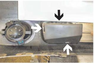
**15.** Set fascia face down on a soft surface, release the three clips on grill cap and remove cap, both sides. Grill caps will not be reinstalled.
