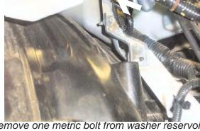
**8.** Remove one metric bolt from washer reservoir's upper bracket using the 10MM socket.
