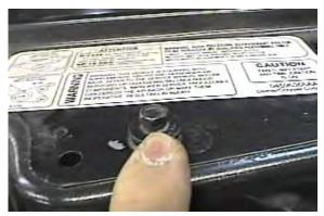
3. Remove the two metric bolts on the top side of the grill with 10MM socket. Pull fascia forward and set aside.
