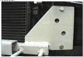
8. Hold baseplate in place so that top edge of end plates are flush with top frame webbing. Using the baseplate as a template, drill four holes on the front side of baseplate with the 13/32 drill bit. Insert items 3, 4, and 5, do not tighten.
