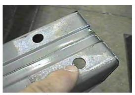
10. Drill out the four mounting holes on the back side of metal bumper with a 13/32 drill bit. Install items 6, 7, and 8 with metal bumper and tighten all bolts. Be sure and use loctite on all bolts before tightening.
