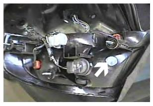
**Note:** If installing the BX8869 bulb and socket wiring kit, this is the recommended location for drilling the hole.
