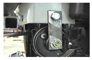
14. Reinstall horn using bracket provided, item 9. Be sure to use loctite on all bolts before tightening.
