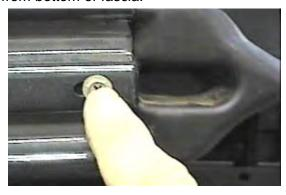
**4.** With a phillips screw driver remove screw metal bumper ends. Remove end caps and set aside.
