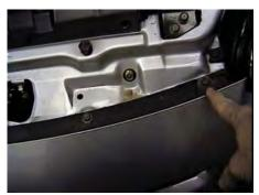
**1.** Using the 10MM socket, remove the five metric bolts from the top side of fascia.
