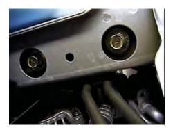
5. Remove two metric bolts from the bottom side of frame rails using the 14MM socket, both sides. Pull metal bumper forward and set aside.
