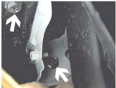
6. Pull plastic back just forward of front tires and remove two metric bolts from back side of fascia's corner with the 10MM socket, both sides.
