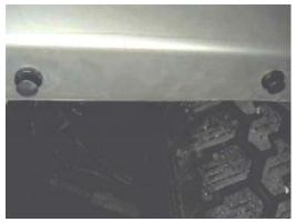
8. Remove four push pins from bottom edge of front fascia, just under belly pan and two just forward of front tires on the bottom edge of fascia, both sides.
