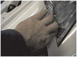
3. Just inside of head lights pull grill forward to release on both sides, lift up and set aside.
