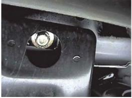
7. Using the 12MM socket, remove two metric bolts from the front of the belly pan, loosen the two back metric bolts and set aside.
