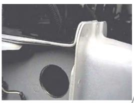
**12.** Drill one hole in frame on the outer side next to sensor, using the 1 1/4" hole saw, both sides.
