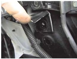
**11.** Bend brackets up on both sides to open area for baseplate insertion.
