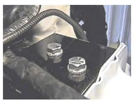
14. Using the baseplate as a template, drill the two remaining holes on the top of frame rails with the 13/32" drill bit, each side. Insert nut plates into 1 1/4" drilled hole to align with these drilled holes, tighten 3/8" bolt and lock washer, both sides. Be sure to use loctite on all bolts before tightening. Tighten all bolts according to Torque Chart in General Instruction Sheet.
