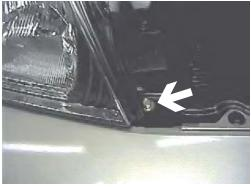
**4.** Remove three metric bolts from the top of metal bumper between headlights with the 10MM socket.
