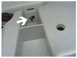
2. Release the four clips on the top edge of fascia just under plastic in step 1.
