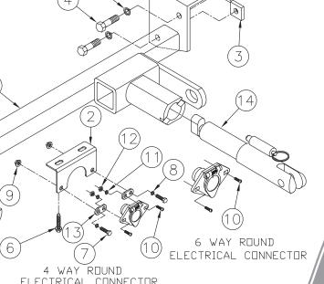
IMPORTANT: Use only genuine factory replacement parts on your Base Plate. Do not substitute homemade or nontypical parts. If a bolt is lost or in need of replacement, for your safety and the preservation of your Base Plate, be sure to use a replacement bolt of the same grade (Usually Grade 5, refer to parts list). Repair parts may be ordered through your nearest *Blue Ox* dealer or distributor.
