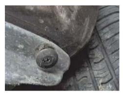
**5.** On bottom edge of fascia are eight push pins to remove, pull fascia forward and set aside.
