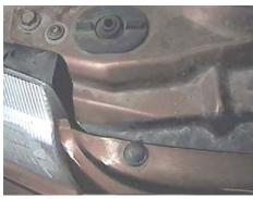
**2.** Just between headlights, on fascia's edge, are five push pins to remove.
