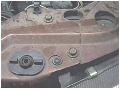
Remove two torx bolts from the top side of headlight assembly with the T-30 torx, pull assembly forward, unplug electrical connections, and set aside, both sides.
