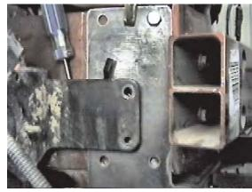
7. Using the baseplate as a template, drill the four holes with the 13/32" drill bit, both sides. Insert 3/8-16 x 1" bolt through baseplate into drilled hole and tighten hex nut and lock washer, according to drawing on page 3, both sides. Be sure to use loctite on all bolts before tightening. Tighten all bolts according to Torque Chart in General Instruction Sheet.
