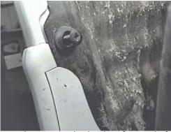
**5.** Remove the two push pins just forward of the front tire on fascia's edge, both sides.
