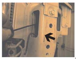
12. Drill out existing hole and drill all the way through to the back side of radiator cross member, both sides. Be sure there is nothing behind cross member before drilling.
