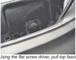
2. Using the flat screw driver, pull top fascia's edge back to expose and remove two push pins that release inner fascia's brace.
