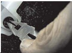
**8.** Remove two push pins from tabs on lower fascia's edge using the needle nose pliers.
