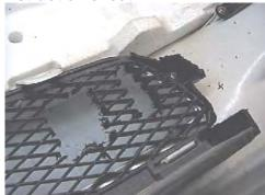
**17.** Hold fascia to align with its original position. Using the utility knife mark and trim lower grill to allow baseplate to come through.
