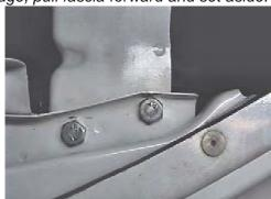
11. Drill one hole in bumper bracket on top of frame, one in bumper bracket and webbing. Insert 3/8" hex nut and lock washer into frame opening to align with drilled hole and tighten 3/8-16 x 1 bolt. Align 3/8" hex nut and lock washer with hole on the bottom side of webbing, tighten 3/8-16 x 1" bolt. Be sure and use loctite on all bolts before tightening. Torque all bolts according to the torque chart in the General Instruction sheet.
