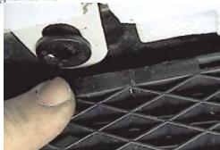
7. Push grill back to expose and remove two push pins from lower opening with the needle nose pliers (see photo step eight).
