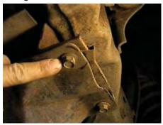
Remove forward metric bolt from cross member, on the bottom of frame, with the 13MM socket and remove nut clip from cross member, both sides.
