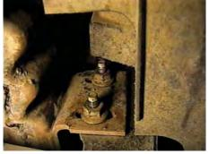
2. While holding bumper in place, remove two metric nuts from the back side of bumper, using the 21MM socket, both sides.
