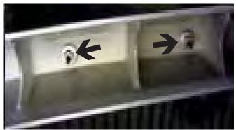
2. Remove the six hex nuts on the back top edge of the fascia with 11MM socket. Pull the front chrome grill forward and set aside.
