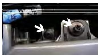
**3.** Just behind the head light assemblies are three metric bolts to remove using an 8MM socket, both sides. Pull assemblies forward and set aside, both sides.
