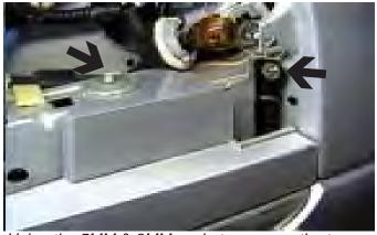
**5.** Using the 5MM & 8MM sockets, remove the two hex head screws from blinker opening on each side.
