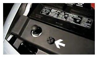
1. Unscrew 3 pins from black plastic on the top edge of fascia ,lift up and set aside.
