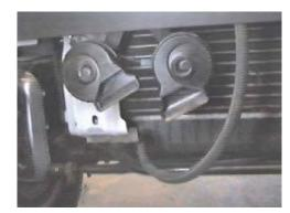
2. Remove two metric bolts from back side of horn assemblies with the 10MM socket, unplug electrical and set aside.
