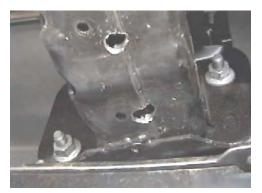
1. Remove two push pins from plastic belly pan and set aside. Using the 21MM socket, remove four metric bolts from the back side of the metal bumper and set bumper aside.
