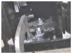
3. Slide baseplate from the bottom up to the frame and clamp in place with the vise grip, both sides. Using the baseplate as a template, drill the two bottom holes with the 17/32" drill bit, both sides. Insert 1/2" hex bolts into baseplate and drill holes, tighten 1/2" lock washer and hex nut. Be sure and use loctite on all bolts before tightening. Tighten all bolts according to torque chart in the General Instruction sheet.
