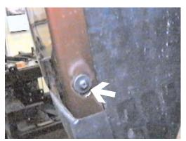
**5.** Remove the two phillips screw just forward of the front tire, on fascia and wheel well edge with the phillips screw driver, both sides.
