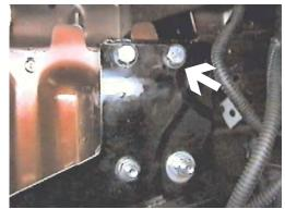
14. Using the baseplate as a template drill two remaining holes into webbing on the top edge of frame with the 13/32" drill bit, both sides. Insert 3/8" hex bolts into baseplate and drilled holes. Tighten 3/8" hex nuts and lock washers according to drawing on last page, both sides. Be sure and use loctite red on all bolts before tightening. Tighten all bolts according to Torque Chart in General Instruction Sheet.
