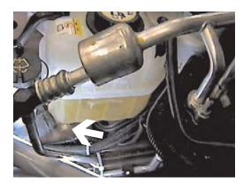
11. Remove the metric bolt just under radiator reservoir and behind headlight assembly with the 8MM socket, disconnect electrical and fluid hoses, set aside.
