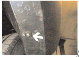
**6.** Just forward of front tires and on fascia's lower edge are nine phillips screws to remove with the phillips screw driver, both sides.
