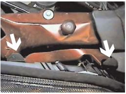
2. Pull the two clips straight up just behind headlight assembly, pull forward, unplug electrical and set aside, both sides.
