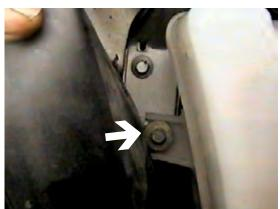
**11.** Using the 10MM socket, remove one metric bolt from air baffle on passenger's side.
