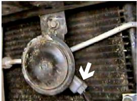
7. Unplug electrical connections to horns attached to lower metal bumper and pull connectors out of the way.
