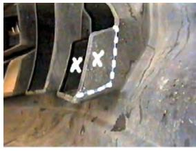
20. Using a utility knife, cut and remove the marked pieces from the back side of fascia, both sides.
