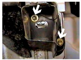
**8.** Remove two metric bolts from metal bumper, both sides using the 13MM socket, pull forward and set aside.
