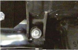
7. Using the 10MM socket remove the lower metric bolt from the air baffle, on the driver's side. Disconnect the hose clamp, pull baffle down to unsnap from top bolt and set aside.
