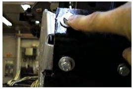
9. Remove the two metric bolts from outer frame end cap and align front holes of item 2 with the frame holes on driver's side, insert bolts and tighten. Using item 2 as a template drill the four remaining holes into frame with the 13/32" drill bit. Remove item 2 from frame. Repeat process for passenger's side and item 3.
