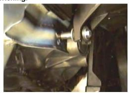
14. Reinstall air baffle on driver's side using items 6 and 18 on the lower bolt. Reconnect hose clamp. Be sure and use loctite on all bolts before tightening.
