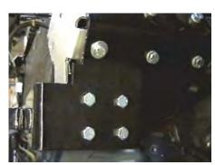
13. Align item 1 on the outside of items 2 and 3 holes, install items 9, 11, 12, and 13 according to drawing on page 4. Tighten all bolts on items 1, 2, 3 and 4. Trim air dam as needed to relieve area for item 1. Be sure and use loctite on all bolts before tightening.
