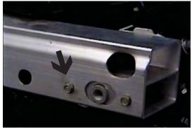
5. Remove the two metric bolts with the 10MM socket and set tow bracket aside.
