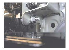
13. Install 3/8" bolt lock washer and hex nut into lower hole on both sides. Be sure and use loctite on all bolts before tightening. Torque all bolts according to torque chart in the General Instruction sheet.
