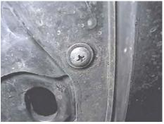
**4.** Using the phillips screw driver, remove two screws from bottom edge of fascia just forward of front tires, both sides.
