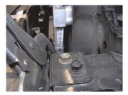
**9.** Remove two metric bolts from the top and one metric bolt from the bottom of the metal bumper using a 13MM socket, both sides. Pull bumper forward and set aside. 2003 Model will need to use a 12MM socket.
