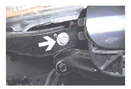
**7.** Remove two metric bolts from the lower head light assembly with the 10MM socket, both sides. Pull head light assemblies forward, unplug and set aside.
