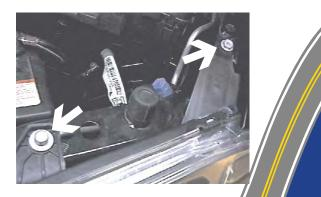
Using the 10MM socket, remove two metric bolts from head light assembly.
