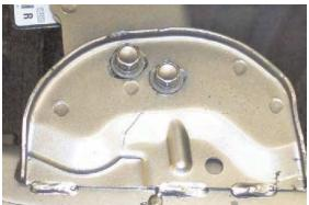
7. Using the 12MM socket, remove metric bolt from the top side of metal bumper, both sides.
