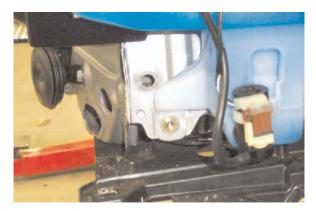
**9.** Remove the three metric bolts from washer reservoir using the 10MM socket, unplug electrical connections, disconnect and plug water lines, set aside.
