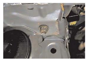
**8.** Remove one metric bolt from the bottom side of metal bumper using the 12MM socket, pull forward and set aside.
