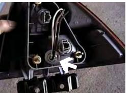
Location for the BX8869, bulb and socket on the driver's side of the 2004 model.
