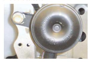
**10.** Using the 12MM socket, remove the metric bolt from horn bracket on driver's side.
