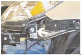
6. Remove the metric bolt from headlight assembly with the 10MM socket, pull forward, unplug electrical and set aside, both sides.
