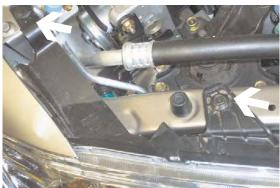
**4.** Using the 10MM socket, remove one metric bolt and one push pin from the top side of headlight assembly, both sides.
