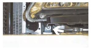
**5.** Remove one metric bolt from below headlight assembly with the 10MM socket, both sides.
