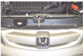
Remove the eight push pins from black plastic cover on top side of fascia, lift cover and set aside.
