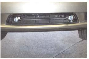
17. Hold fascia to it original position and trim horizontal rib to allow attachment receivers to come through. OPTIONAL METHOD: Remove lower black plastic from the back side of fascia's opening.
