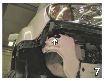
7. Remove this bolt on the side. Do this to both sides of the vehicle. Set bolts aside to reinstall later.
