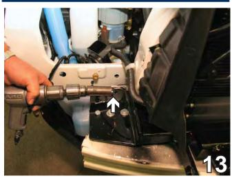
13. Temporarily slide the metal bumper in between the frame and the baseplate. Insert additional bolts and tighten using Loctite. Torque to specs. Do this on both sides. Drill the side hole being sure not to drill into the radiator, use a socket over the drill bit.
