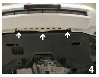
Using a 10MM socket, remove three metric bolts that run horizontally along the bottom of fascia, where the belly pan and fascia meet. Set bolts aside to be reinstalled later.
