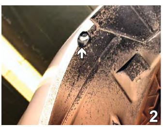
2. Just forward of the front tire, on the edge of the fascia, use an 8MM socket or Phillips screwdriver to remove one metric bolt. Set bolt aside to reinstall later. Do this to both sides of the vehicle.
