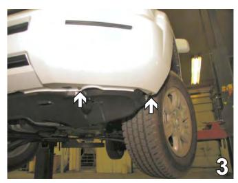
3. Just forward of the front tire, on the outermost bottom edge of fascia, remove two metric bolts using a 10MM socket. Do this to both sides of the vehicle. Set bolts aside to reinstall later.
