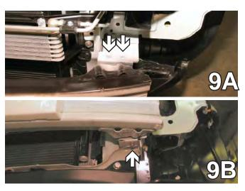
Using a 12MM socket, remove two metric bolts on the top and one metric bolt underneath the metal bumper. Do this to both sides of the vehicle. Set bolts aside to reinstall later.
