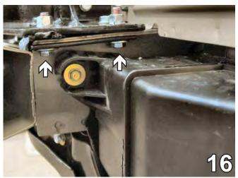
16. Place the backing plate on the bottom side of the frame webbing to align with drilled holes, insert the 3/8-16 x 1 1/2" hex bolts and 3/8" flat washers into this hole, tighten the 3/8-16 hex nuts and 3/8" lock washers. Reinstall the air baffle to its original position.
