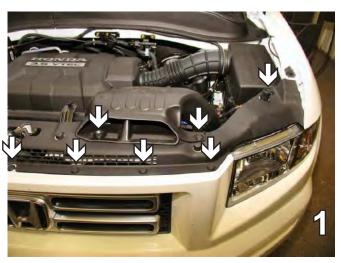
1. Remove 12 pushpins from the plastic above the radiator. Remove the plastic from the top of the radiator. Set pushpins aside to reinstall later.
