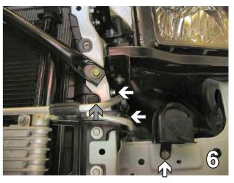
6. Remove another push pin from underneath, gray arrow. Remove the two bolts on the side. Using a 12MM socket, remove the bolt from the horn bracket, bottom arrow. Do this to both sides of the vehicle. Set push pins and bolts aside to reinstall later.
