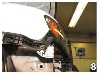
Using a Phillips screwdriver, remove the screw. Do this to both sides of the vehicle.
