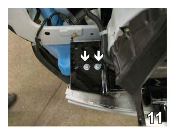
11.Slide metal bumper back on to the frame rail, guiding the baseplate on top of frame rail. Align with the existing holes of the bumper bracket. Insert two 8MM-1.25 x 30MM hex bolts through the baseplate into the two existing bumper bracket holes using 5/16" lock washer and 5/16" flat washers Snug the bolts down. Do this on both sides.
