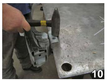
Lay the bracket of the metal bumper on a solid surface. Use a hammer to pound and flatten the rib on top of the bracket. Do this to both sides of the vehicle.
