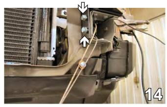
14. Remove metal bumper. Insert the 3/8-16 hex bolts with the 3/8" lock washer through the baseplate holes on the side of the frame rail. Hand tighten bolts to the 3/8-16 nut plates placed on hex bolts through opening in frame end. Do this to both sides of the vehicle. Using diagonal cutters, cut all nut plate wires flush with the end of the frame. Reinstall bumper and tighten bolt for steps 12, 13 and 14. Be sure to apply LOCTITE Red to ALL bolts.
