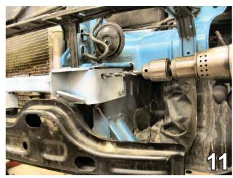
11. Using the baseplate as a template, drill the two remaining holes with the 13/32" drill bit. Do this to both sides of the vehicle.
