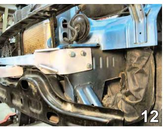
12. Insert the 3/8" nut plates into the opening on the end of the frame to align with drilled holes. Tighten the 3/8" lock washers and the 3/8-16 x 1 1/2" hex bolts into the nut plates., Do this to both sides of the vehicle.
