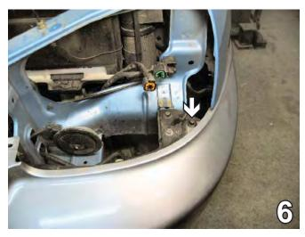
5. Just below headlight assembly is a Phillips pushpin to remove. Do this to both sides of the vehicle. Set pushpins aside to be reinstalled later. Pull fascia corner out to the side and then forward. Unplug marker lights and unplug fog light, if applicable. Set fascia aside to be reinstalled later.
