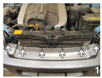
Remove six Phillips pushpins from the top edge of the fascia. Set pushpins aside to be reinstalled later.
