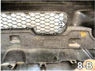
8. Set the front fascia face down on a soft surface to protect it from being scratched. Using a small flat screwdriver, release the sixteen clips from the grille, shown in 8-A. Remove the side clip from the fascia with a utility knife 8-B. The **GRILLE** will **NOT** be reinstalled.
