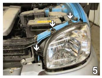
5. Using the 10MM socket, remove the three metric bolts from the headlight assembly. Pull assembly forward and unplug electrical connections. Do this to both sides of the vehicle. Set headlight assemblies and metric bolts aside to be reinstalled later.
