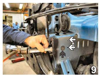
9. Remove the two weld nuts from the existing holes inside the frame with the Flat Cold Chisel, see grey arrow in the photo above. Remove the rubber plug from the frame, please reference the white arrows in the photo above. Do this to both sides of the vehicle. Plugs will NOT be reinstalled.
