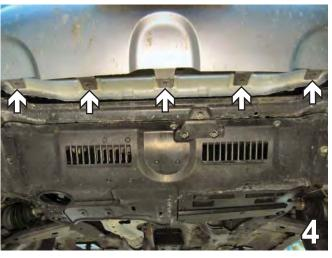
Remove the five metric bolts from the lower edge of the front fascia with the 10MM Socket. Set bolts aside to be reinstalled later.
