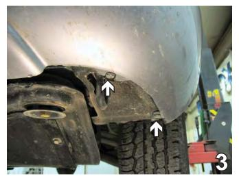
Remove the two Phillips screws just forward of the front tire, on the underside of the fascia, with the Phillips screw driver. Do this to both sides of the vehicle. Set screws aside to be reinstalled later.
