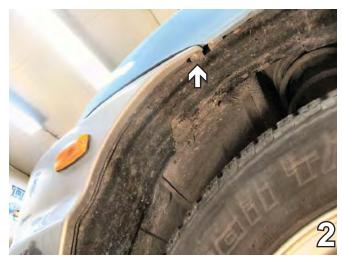
Just forward of the front tire is one Phillips screw to remove with the Phillips screwdriver. Do this to both sides of the vehicle. Set screws aside to be reinstalled later.
