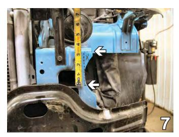
7. Mark two horizontal lines, one 3 3/4" and one 5/8" down from the top edge of frame's front edge. Mark a vertical line flush with the outside edge of the frame. Remove this area with the Reciprocating Saw. Do this to both sides of the vehicle. Using a good quality paint, spray all cut edges of the frame to prevent rusting.
