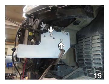
15. On the driver's side, insert 3/8-16 nut plates through frame end hole. Align to the lower two drilled holes (see white arrows). Install 3/8-16 x 1 ½" hex bolts with 3/8" lock washers and tighten. Trim excess nut plate wire. Remove air bag sensor bolt (see grey arrow).
