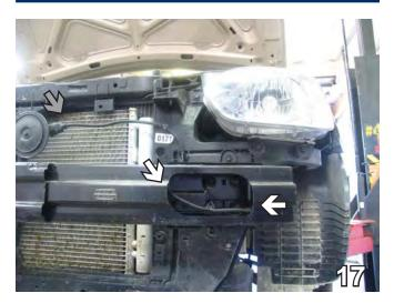
17. Reinstall metal bumper and bracket. Route the horn cable through the side of the metal bumper and out through backside of the metal bumper (see white arrows). Connect the horn cable (see grey arrow).
