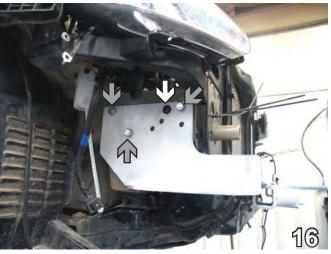
16. On the passenger's side, align baseplate with washer reservoir hole and insert existing bolt (see white arrow). Using the baseplate as a template, drill three holes into the frame rail with the 13/32" drill bit (see grey arrows). Insert 3/8-16 nut plates through frame end hole. Insert 3/8-16 x 1 1/2" hex bolts and 3/8" lock washers and tighten to nut plates. Trim nut plate wires. Remove washer reservoir bolt.
