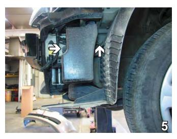
5. On the driver's side, use the 10mm socket to remove two metric bolts from the air baffle. Set bolts and air baffle aside to be reinstalled later.
