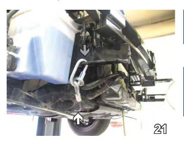
Be sure that **ALL** electrical connections are plugged in properly and functioning **BEFORE** installing the fascia.
