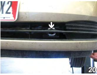
20. Align the fascia to its original position and, using a hack saw blade, trim necessary openings in the grille for the attachment tabs. Do this to both sides of the vehicle.
