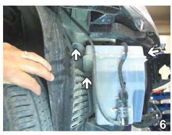
On the passenger's side, disconnect the hose and electrical connection from the washer reservoir. Using the 10mm socket, remove three metric bolts from the washer reservoir. Remove washer reservoir. Set bolts and reservoir aside to be reinstalled later.
