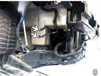
8. On the passenger's side, remove the electrical grounds (see white arrows) and move out of the way for baseplate installation.
