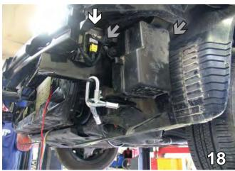
18. On the driver's side, reinstall air baffle's existing bolts to upper rear and lower middle baseplate holes (see grey arrows). Reconnect horn cable to air bag sensor. Reinstall sensor to the top front baseplate hole and insert sensor pin to lower front hole. Reconnect electrical grounds with the 6mm hex bolt and 1/4" lock washer (see white arrow).
