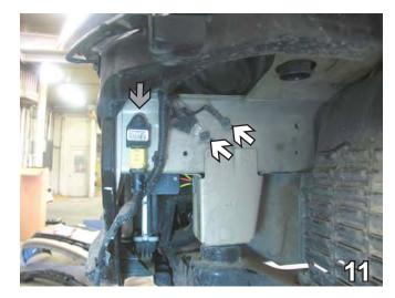
11. On the driver's side, remove the electrical grounds (see white arrows) and move out of the way for baseplate installation. Using the 6mm socket, remove the metric bolt from the air bag sensor (see grey arrow) and move sensor out of way. Set bolt aside to be reinstalled later.
