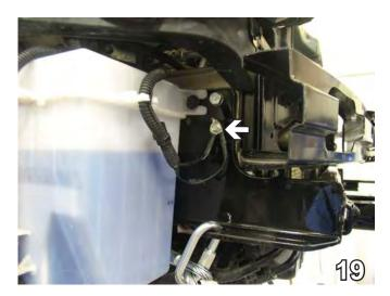
19. On the passenger's side, reinstall washer reservoir using existing bolts. Reconnect electrical grounds to the lower front bolt hole using the #10-16 x 1 self drilling screw (see white arrow).
