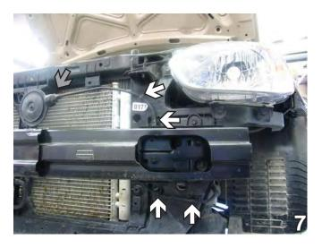
7. Just above the center of metal bumper, press the clip on the horn cable to release it (see grey arrow). Disconnect the cable from four tie clips along the horn cable - between the horn and the air bag sensor on the driver's side. Move the cable out of the way to prepare the area for baseplate installation (leave cable connected to the air bag sensor and move out of the way to prepare area for baseplate installation).
