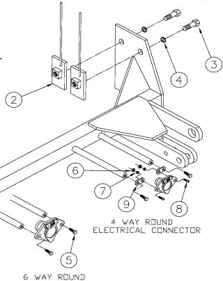
**IMPORTANT:** Use only genuine factory replacement parts on your Base Plate. Do not substitute homemade or nontypical parts. If a bolt is lost or in need of replacement, for your safety and the preservation of your Base Plate, be sure to use a replacement bolt of the same grade (Usually Grade 5, refer to parts list). Repair parts may be ordered through your nearest **Blue Ox** dealer or distributor.
