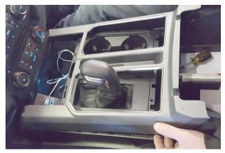
3. Turn key to "Accessories" then shift into "D" (Drive) so you can remove console frame. Then pull frame backwards and up to remove it completely.
