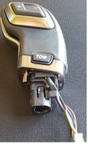
6. Press tabs on shifter base to remove it from boot.
