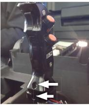
8. Set **shift handle body (1)** down onto factory shifter stem then install screws (removed step 5) into it.
