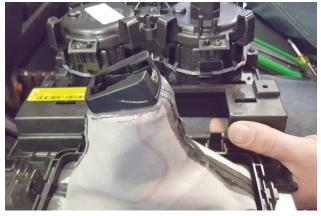
7. Remove shifter collar from boot being careful not to tear cloth material.
