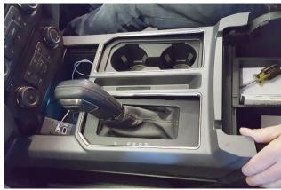
2. Open center console lid then lift and release console frame around shifter.
