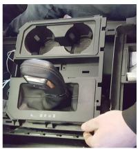
4. Loosen and retain screws (x2) securing cupholder, then lift and release but do not completely remove it from console.
