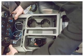
13. Place console frame back into place and snap it down into position. Set shifter back into "P" (Park).
