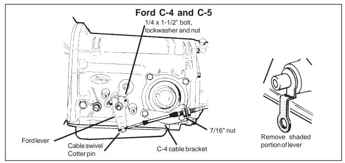
shift lever. If your transmission is so equipped, remove the two bolts holding the switch in place and slide it off the shift shaft. Disconnect the switch at the factory plug and discard it.
