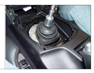
STEP 22. Reinstall shifter cover and bolts. Caution- do not over tighten these bolts. Reinstall center console and console side plates (370Z/G37) if they had been removed.
