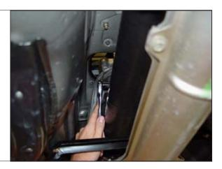
STEP 11. Remove shifter from car. (metal plate and spring will be used on new shifter)
