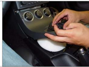
STEP 24. Reinstall knob. Take care not to screw knob down through shifter boot.
