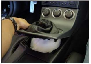
**STEP 3.** Unplug wiring harness from console plate and remove console plate.
