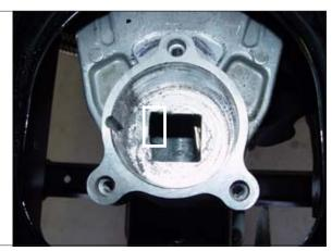
STEP 13. If you were unable to remove the shift knob in step 1, then carefully place the knob in a vise (shifter inverted) and using the long extension or other long tool through the lower connection hole, carefully rotate (unscrew) the shifter assembly off of the shift knob.
