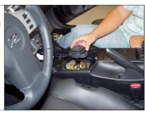
**STEP 7.** Remove bolts holding down metal shifter plate. TOOLS: Socket(10 mm), Drive, and Extension.
