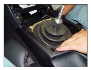
**STEP 23.** Reinstall white foam (350Z and G35 only) and console plate, making sure to replug in wiring harness.
