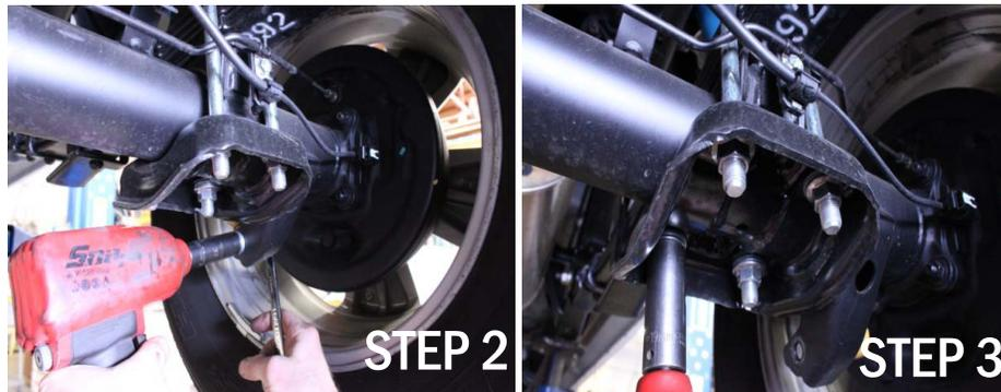
3. Use the floor jack to lift the rear axle, keeping the pin aligned with either the centered hole or the offset hole, and install the new u-bolts with the provided hardware.
