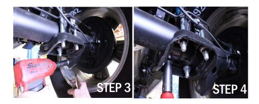
3. Use the floor jack to lift the rear axle, keeping the pin aligned with either the centered hole or the offset hole, and install the new u-bolts with the provided hardware.
