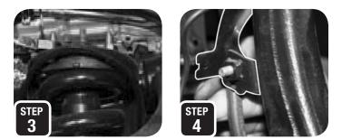
**<u>STEP 4</u>**: Next, remove the clip at the upper ball joint nut, loosen the nut but do not remove, and break the ball joint loose by hitting the side of the spindle with a hammer. The nut will catch the spindle, then remove the nut *(never hit the ball joint on the threads)*.
