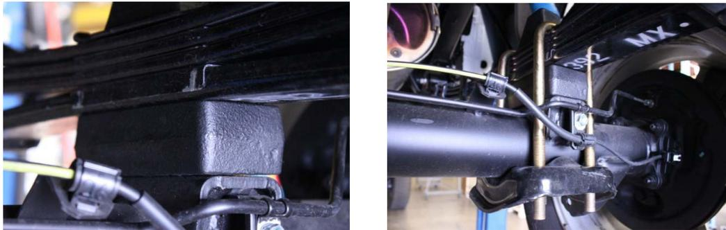
4. Repeat steps on the other side. **NOTE: AFTER, ENSURE THERE IS ENOUGH SLACK IN BRAKE LINES, ABS LINES, AND E-BRAKE CABLES. IF ANY OF THESE ARE TOO TIGHT, MAKE ADJUSTMENTS TO ENSURE THEY ARE NOT STRETCHED WHEN THE AXLE DROOPS OUT.**
