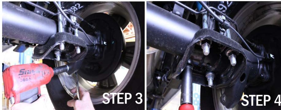
3. Use the floor jack to lift the rear axle, keeping the pin aligned with either the centered hole and install the new u-bolts with the provided hardware.
