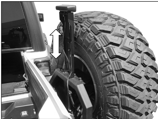
(Fig 29) Swing Arm assembly installed
