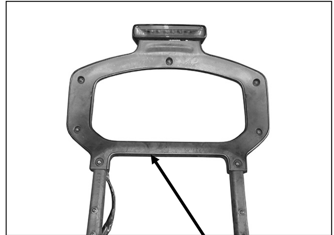
(Fig 26) Remove cover from factory light bracket
