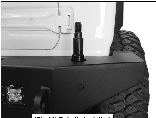
(Fig 11) Spindle installed
