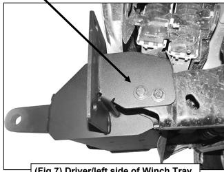
(Fig 7) Driver/left side of Winch Tray
