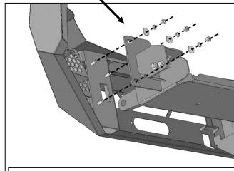
(Fig 16) Attach Bumper to Winch Tray Brackets
