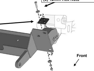
(Fig 9) Attach 3-hole Spacer to top of Hitch Tray
