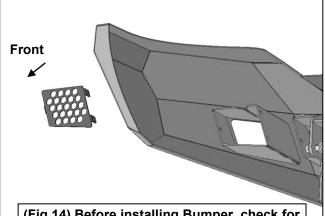
(Fig 14) Before installing Bumper, check for clearance around lights (not included). Remove screens for additional access or to clear lights as needed
