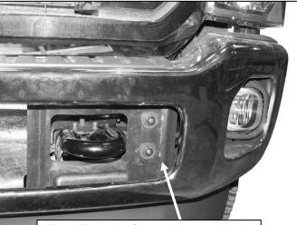
(Fig 3) Remove factory bumper bolts
