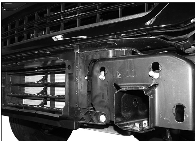
(Fig 3) Remove bumper (driver/left side pictured)
