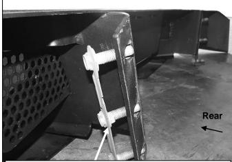
(Fig 4) On models without received hitch, reuse triple bolt plate to attach bumper to ends of frame
