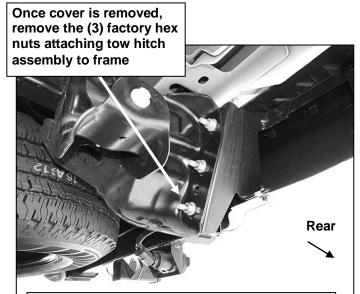
(Fig 3) Remove (3) hex nuts per side to remove bumper reinforcement or receiver hitch
