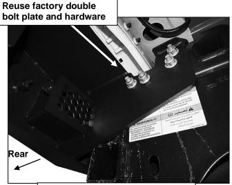
(Fig 6) Reuse factory hardware to attach mounting plate to side of bumper (passenger side pictured)
