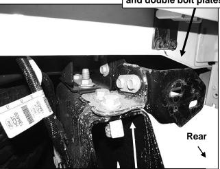
(Fig 4) Remove factory bumper brackets, Do not remove 90-degree support bracket
