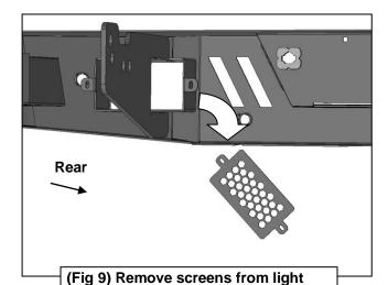
mounts if necessary for additional clearance around or access to lights
