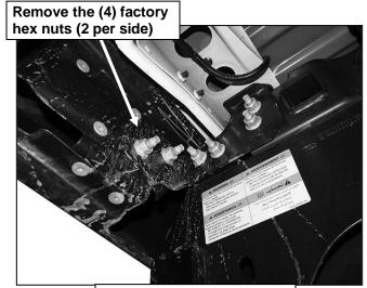
(Fig 2) Remove hex nuts to remove bumper assembly
