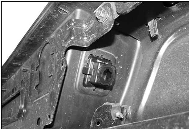
(Fig 5) Disassemble bumper to remove license plate lights, trailer plug, sensors and wiring harness from bumper as equipped
