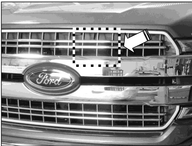
(Fig 1) IMPORTANT: Installation not recommended on 2018-on F150 models with chrome horizontal bar or bars at top of grille (arrow) . The thick, reflective chrome horizontal bars may interfere with sensor operation. NOTE: Lariat model with chrome package pictured. Applies to chrome versions of grille only
