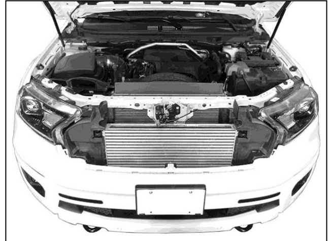
(Fig 21) Ranger Models. Release clips on bottom of grille to remove grille.
