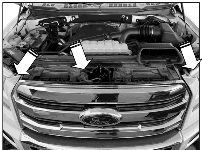
(Fig 2) F-150 Models. Remove cover from top of grille (arrow). Remove hardware attaching top of grille to radiator core support. Release clips attaching top of plastic headlight surrounds (arrows above headlights)
