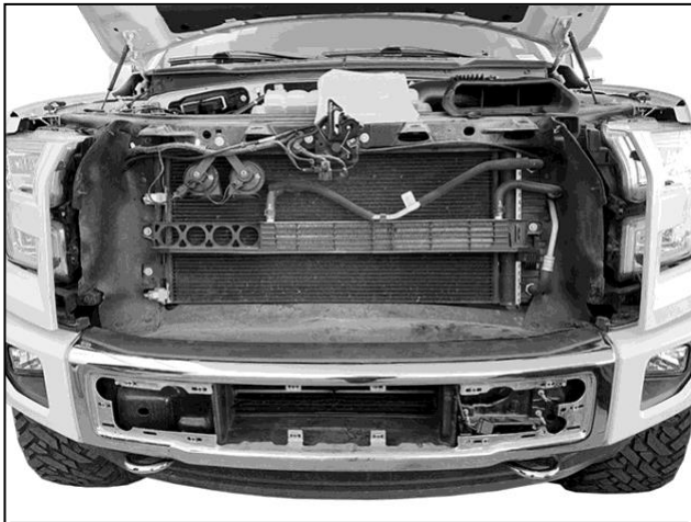
(Fig 4) F-150 Models. Unplug harness leading to shutter in grille. Remove grille assembly
