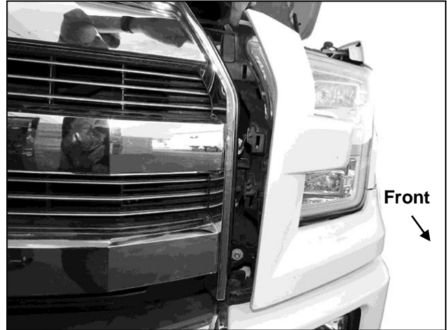
(Fig 3) F-150 Models. Pull out plastic headlight surround to access grille hardware along sides
