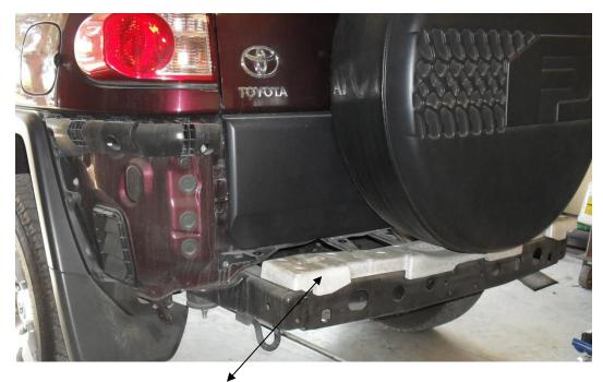
3 Remove Styrofoam center piece.
