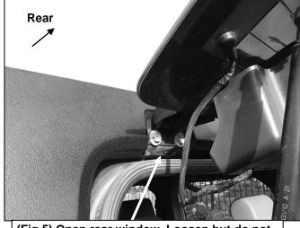
(Fig 5) Open rear window. Loosen but do not remove (2) rear window hinge bolts (arrow)
