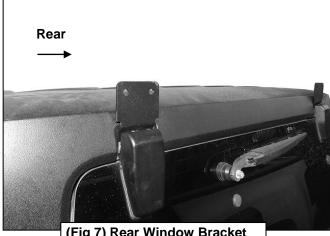
(Fig 7) Rear Window Bracket installed on driver/left side
