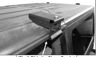
(Fig 4) Slide the Clamp Bracket under the rain gutter (arrow)
