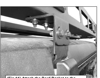
(Fig 11) Attach the Roof Basket to the Rear "L" Brackets (driver side pictured)
