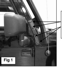
Use the (4) factory hinge bolts to secure passenger side Light Bar Leg
