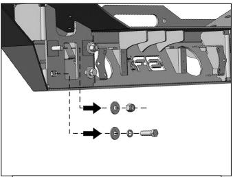
(Fig 7) Temporarily remove the outer bumper bracket support (Fig 2). Do not remove the Bolt/Nut Plate from the Bumper
