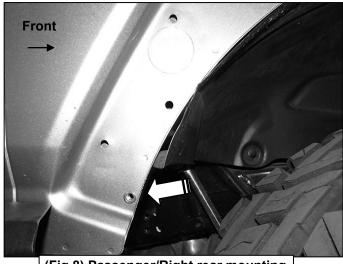
(Fig 8) Passenger/Right rear mounting locations with inserts fully installed
