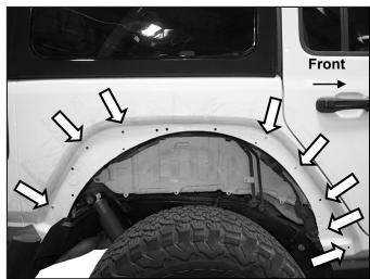
(Fig 4) Drill 25/64 hole in body panel at (8) locations (arrows). NOTE: These locations are not accessible from back of body panel
