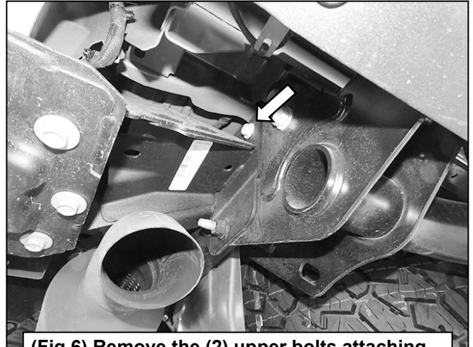
(Fig 6) Remove the (2) upper bolts attaching the rock rail (if equipped) to the receiver hitch
