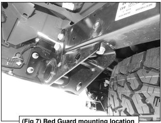
(Fig 7) Bed Guard mounting location (Passenger/Right side shown)
