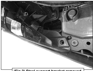
(Fig 2) Steel support bracket removed (Passenger/Right side shown)
