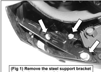
(Fig 1) Remove the steel support bracket from the inner edge of the bumper (Passenger/Right side shown)
