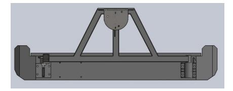
Note: the properly adjusted cam lock will close the carrier tight against the stop and can be latched using one hand with 20 to 25 pounds of force.
