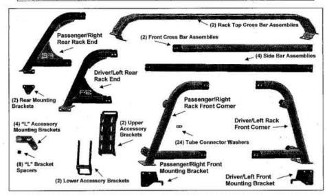
REMOVE CONTENTS FROM BOX. VERIFY ALL PARTS ARE PRESENT. READ INSTRUCTIONS CAREFULLY BEFORE STARTING INSTALLATION. ASSISTANCE IS HIGHLY RECOMMENDED.
